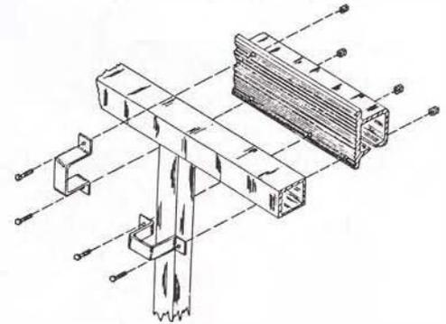
4. BOLTED DIRECTLY TO HORIZONTAL AND/OR VERTICAL FRAMING
